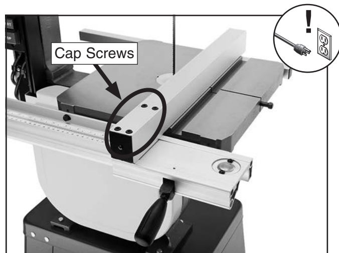
Figure 41. Location of the fence adjustment cap screws.
