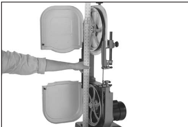
Figure 68. Checking if the wheels are coplanar.
